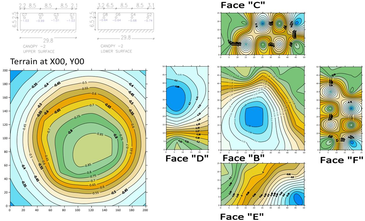
FIGURE 22 Pressure coefficients on terrain and model surface tornado location at 00m.
