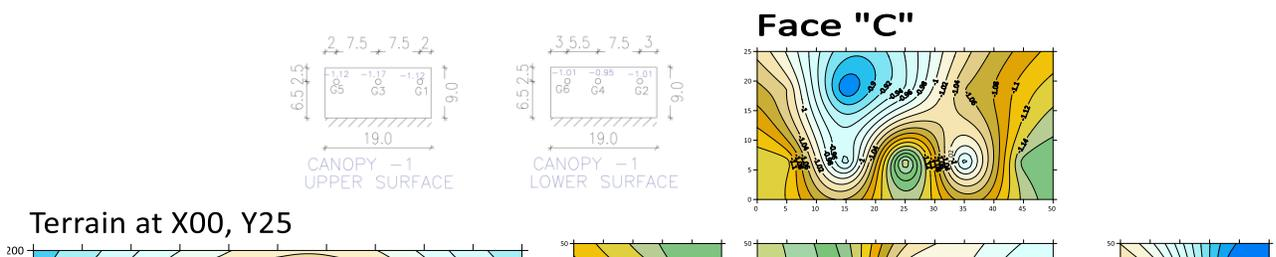
FIGURE 16 Pressure coefficients on terrain and model surface tornado location at 10 m in Y-direction
