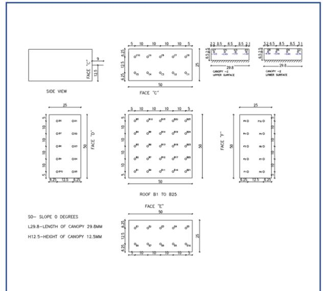
FIGURE 4 | Exploded view of the pressure points of base plate, model surface and canopy
