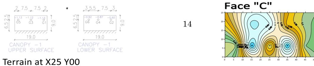
FIGURE 19 Pressure coefficients on terrain and model surface tornado location at 10 m in X-direction
