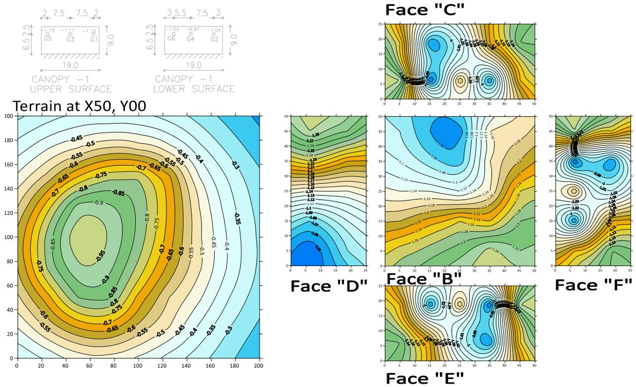
FIGURE 20 Pressure coefficients on terrain and model surface tornado location at 20 m
