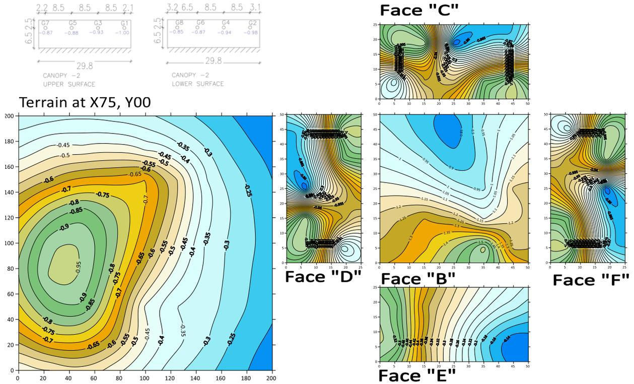
FIGURE 28 Pressure coefficients on terrain and model surface tornado location at 30m in X direction
