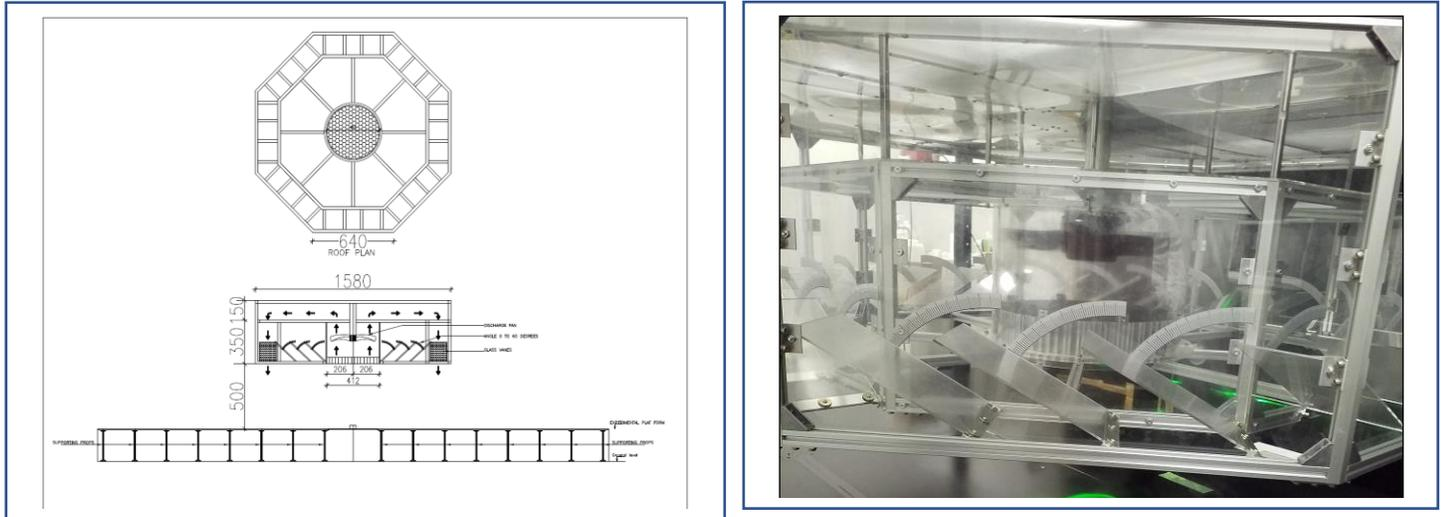
FIGURE 5| Translating tornado-like flow simulator at Tokyo Polytechnic University and schematic showing the dimensions
