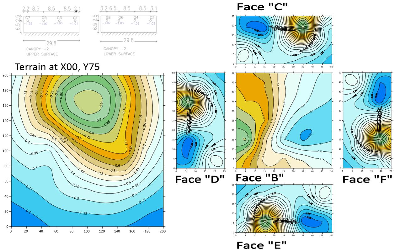
FIGURE 25 Pressure coefficients on terrain and model surface tornado location at 30m.
