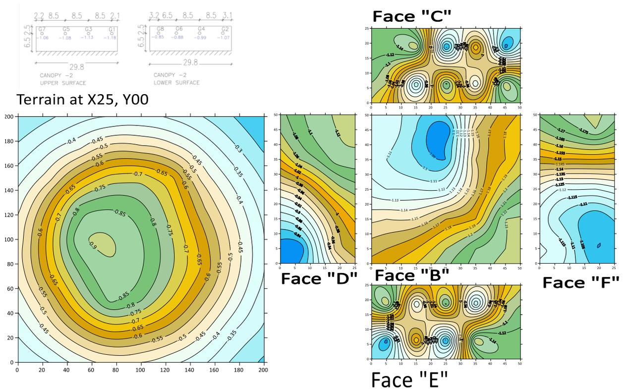
FIGURE 26 Pressure coefficients on terrain and model surface tornado location at 10m in X direction.
