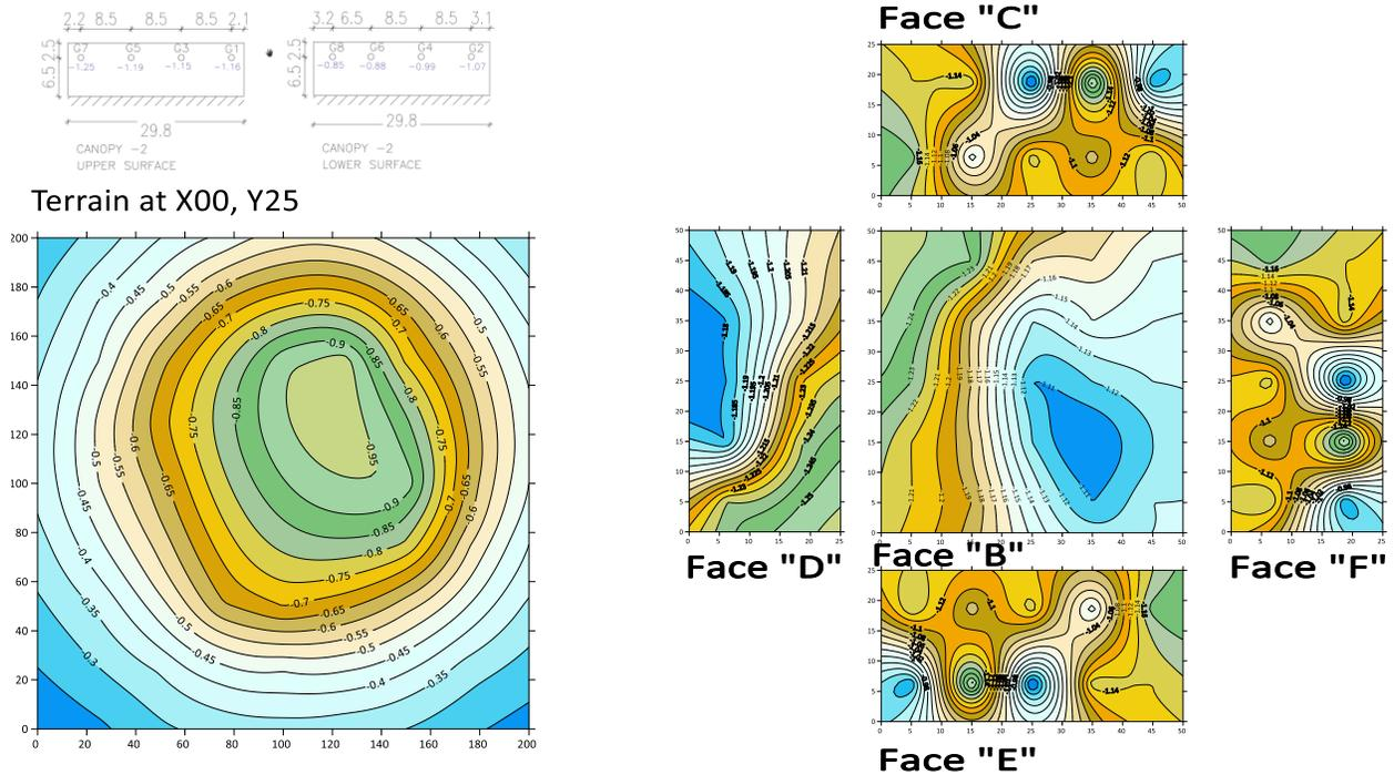
FIGURE 23 Pressure coefficients on terrain and model surface tornado location at 10m.
