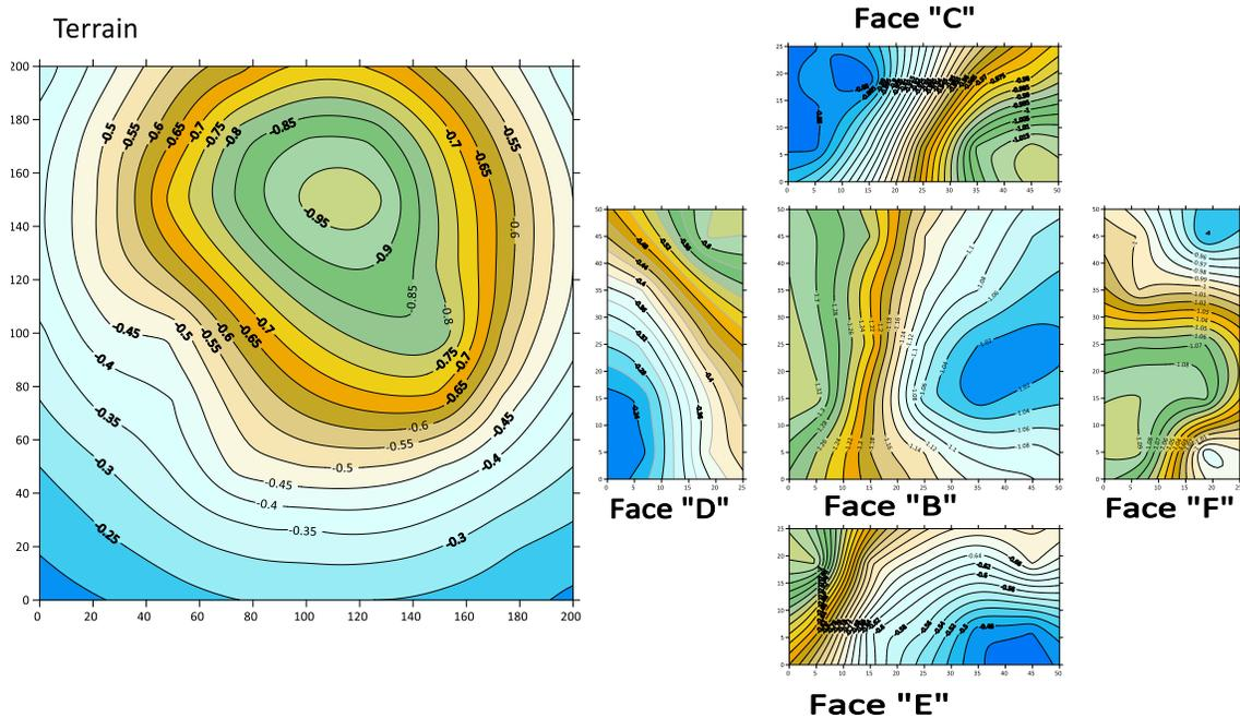
FIGURE 13- Pressure coefficients on terrain and model surface tornado location at 20m.
