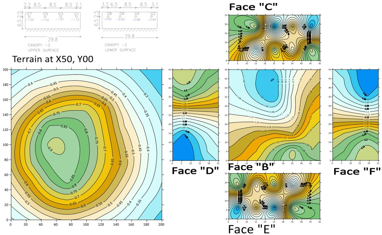
FIGURE 27 Pressure coefficients on terrain and model surface tornado location at 20m in X direction.
