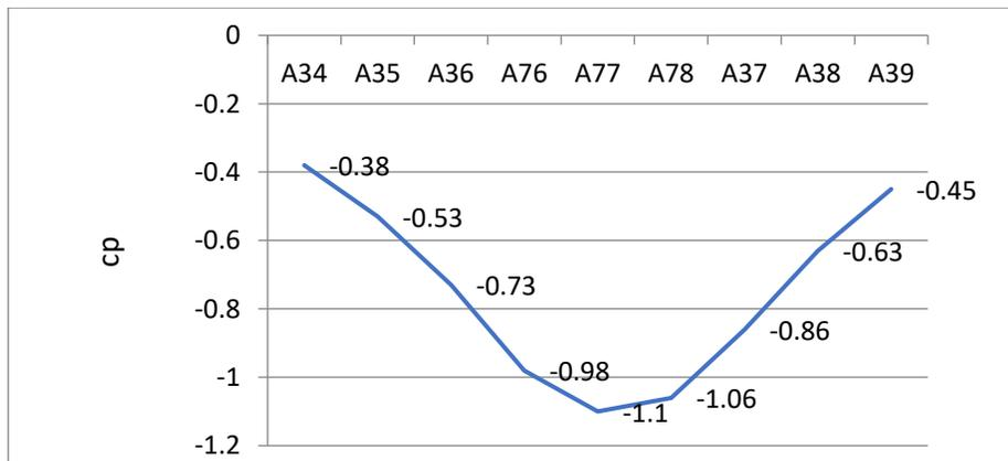
FIGURE 10| Radial distribution of the surface pressure coefficient along the x- and y-direction passing through the center of the stationary tornado.
