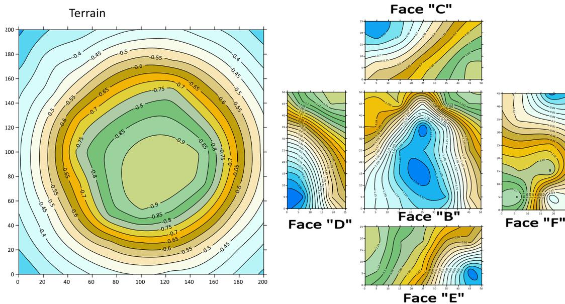
FIGURE 11|– Pressure coefficients on terrain and model surface tornado location at center of model
