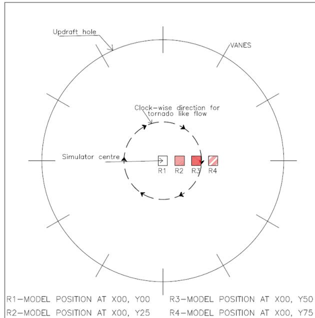
FIGURE 2 Building Model position on simulator floor
