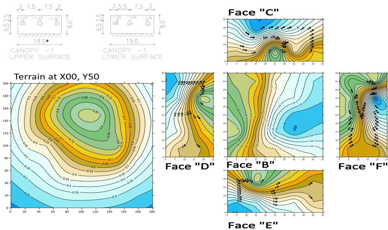
FIGURE 17 Pressure coefficients on terrain and model surface tornado location at 20 m
