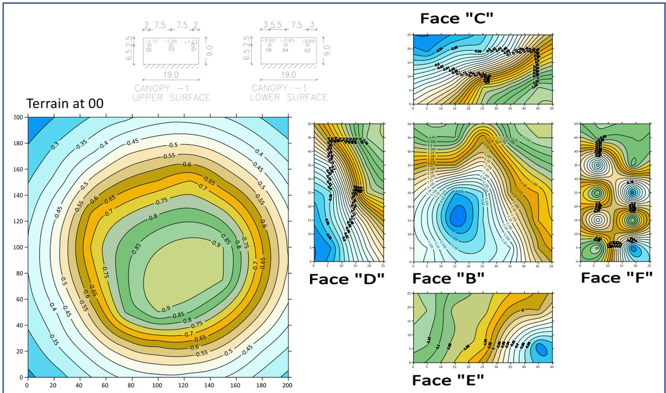
FIGURE 15 Pressure coefficients on terrain and model surface tornado location at 00m.
