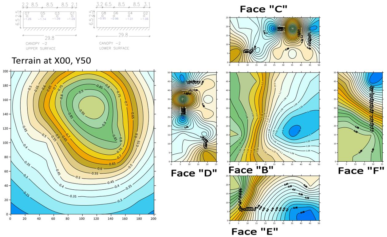
FIGURE 24 Pressure coefficients on terrain and model surface tornado location at 20m.
